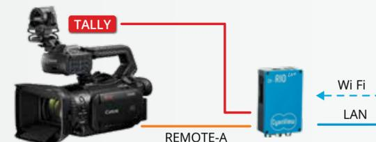
Just like the EOS series, the Remote-A port is used to control Canon camcorders. Tally can be provided as an external light box of LED.
