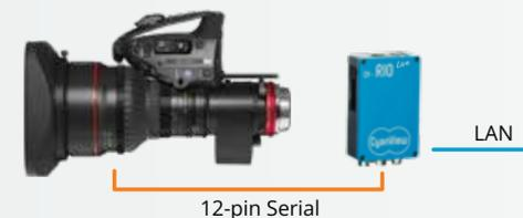
Canon CineServo have the same 12-pin connector as B4 lenses and control is done using the same cable and protocol.
