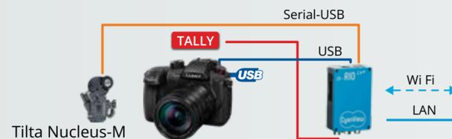
The Panasonic GH5S can be controlled over USB. External lens motors from Tilta or using C-Motion Broadcast Camin are supported. This is useful on gimbals or drones. An external tally box or LED can be connected to RIO directly.
