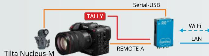
The C70 can also be controlled over Remote-A. An external tally light can be added on the camera hotshoe. Tally motors or C-Motion Broadcast Camin can be used to motorize lenses.
