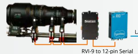
C-Motion supports the “B4 Generic” protocol. You need the C-Motion RVI-9 cable to allow serial control of the unit, and the CY-CBL-6P-B4-01 cable to link it to the RIO connector.
