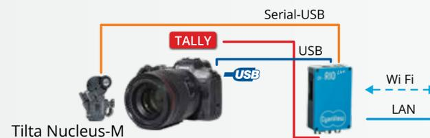
The Canon R5 can be controlled over USB. Control is rather good and bidirectional. Tally motors or C-Motion Broadcast Camin can be used to motorize lenses.
