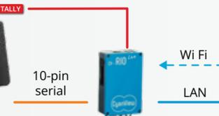
Older P2 camcorders can be controlled using a C10 or Rio Live and a 10-pin adapter cable. Exposure, white/black color balance are available remotely. Some other functions like saturation or menu navigation can be available on some models.
