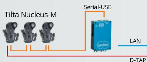
Up to 3 Tilta Nucleus-M Motors can directly be driven by a RIO using the CY-CBL-TILTA-01 USB serial cable. Power is provided on the side from the Tilta D-TAP cable. Calibration of iris range is done through the configuration interface.
