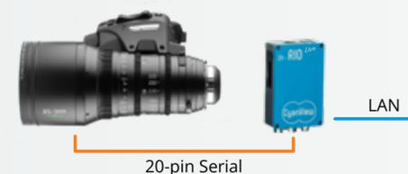
Fujinon lenses can be controlled directly through the 20-pin AUX connector using the CY-CBL-6P-FUJI cable and selecting the protocol named “B4 Fuji” in the interface. It is also possible to use the CY-CBL-6P-B4-01 combined with the Fujinon 20-pin to 12-pin cable and using the protocol named “B4 Generic” in the interface.
