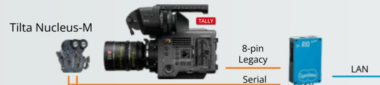
Control of the Venice using a Rio Live which can control the camera over the 8-pin connector and can drive Tilta motors for lens motorization.
