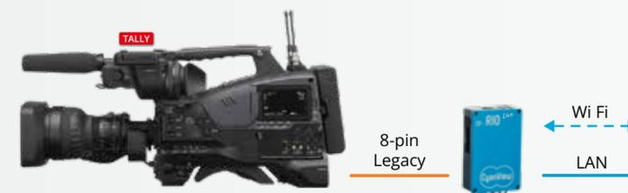
Control of the camera over the 8-pin connector, can be used wired or over wifi. Built-in tally control and all settings provided by the protocol are covered.
