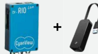
Rio is used to handle multiple interfaces on the camera side like lens control, serial ports, IP or WiFi, and USB. When the camera has a wired IP connection, a USB ethernet dongle can be used in bridged mode to connect both the camera and the inbound connection as if they were on the same switch. It is then still possible to access the camera over its IP address as normal.
