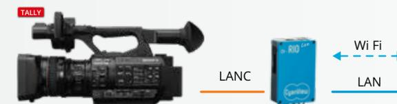
Handheld camcorders can be controlled over LANC. Newer models have built-in tally but an external box or LED can be added. The protocol is limited to exposure (iris, electronic ND, gain), menu navigation, record and tally. No color settings.
