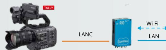
The FX6 and smaller camcorders can be controlled using LANC. The protocol is limited to exposure (iris, electronic ND, gain), menu navigation, record and tally. No color settings unfortunately. The RIO Live can be connected on LAN or Wi Fi
