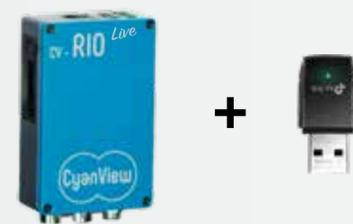
Dual WiFi interface: can create an access point for cameras to connect to it, and connect to another WiFi network at the same time. The Bridged Access Point mode allows accessing connected cameras as if they were on an ethernet switch. This is typically used to keep a very short wifi connection between RIO and the camera and extending it over wired ethernet or fiber.
