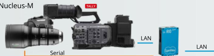
A Rio Live can be added to control ENG or PL lenses directly or through C-Motion or Chrosziel systems, or drive Tilta motors directly.
